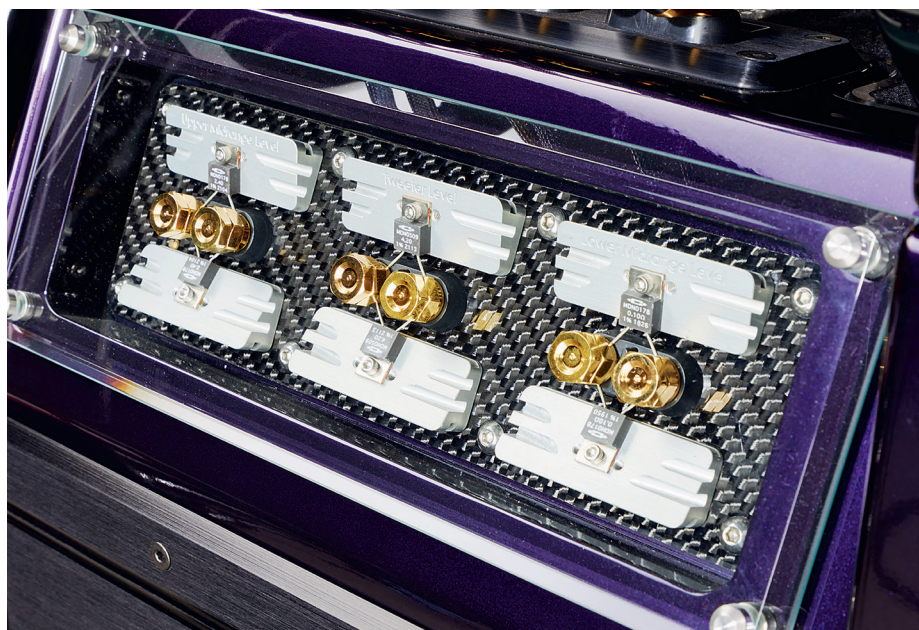
ABOVE: Rear-mounted protection and tuning resistors for the mid and treble drivers are now illuminated, for easy access and visibility. The high-pass mid/treble crossover is also mounted inside the upper section of the bass cabinet
