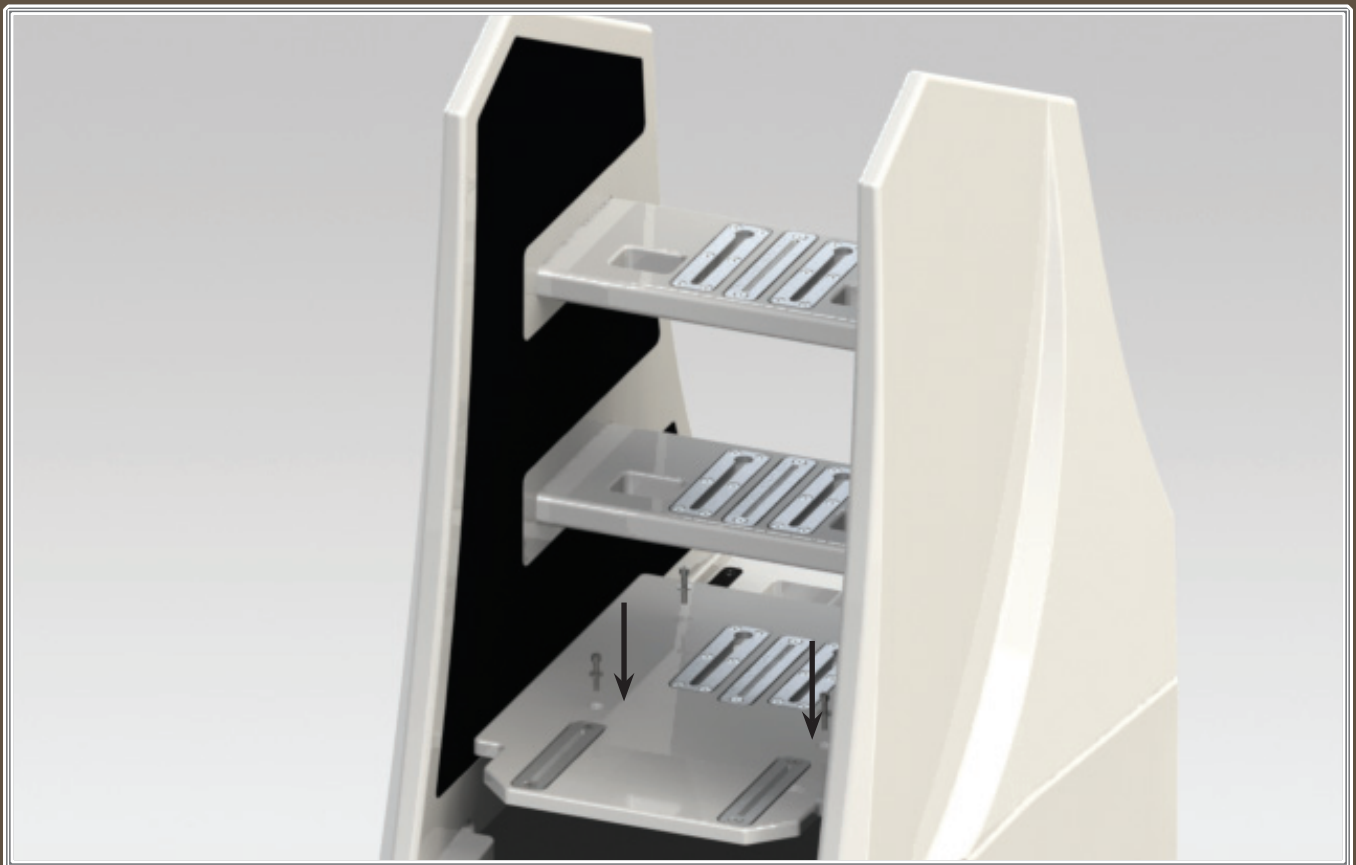
FIGURE 12—REINSTALL PROPAGATION DELAY PLATE AFTER INSTALLING WING.
