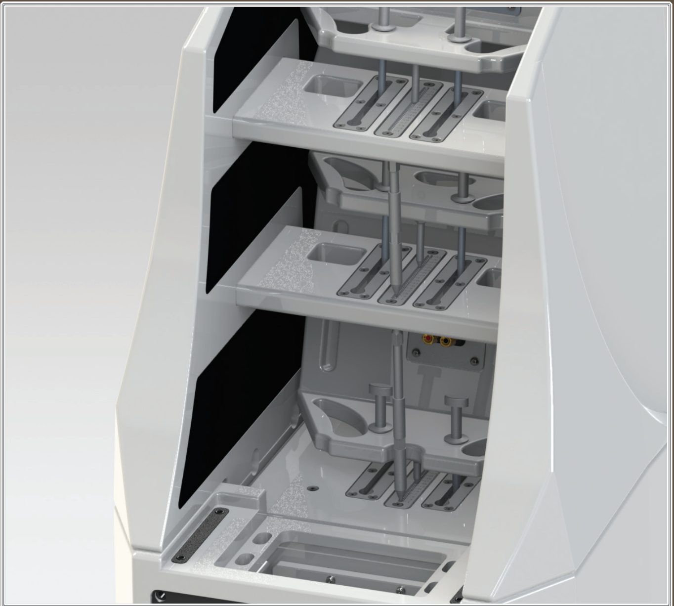
FIGURE 22 - INSTALL THE EXPANSION SPIKES.
