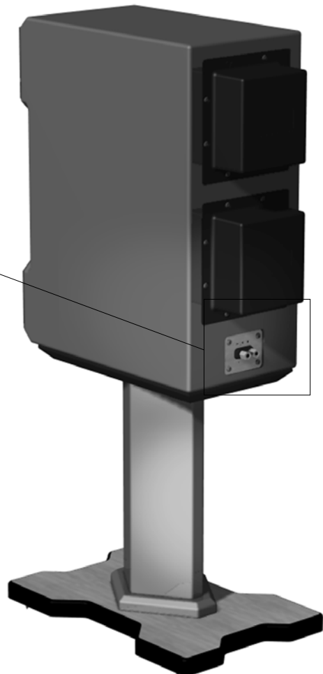
FIGURE 7- CUB CABLE CONNECTION
